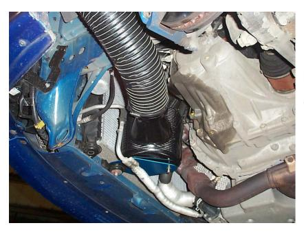
Please remember to use the standard rubber isolator and hold in place with an M8 washer either side before fixing with the M8 Ny-loc nut until compressed.
