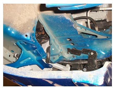
Now refit the bumper in the reverse of how it was taken off and lightly attach the under tray using the three 10mm silver headed (zinc plated) bolts. remembering to fit the metal strap. Fit the two trim clips to the main body (without the centre screw) under drivers' and near side wings. Locate and position the feet correctly and fully through the tray and the receiving hole in the
