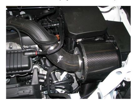
With the top part of the kit fully in place, you now need to tie down the cold air duct into place. There are plenty of places to wrap a cable tie round to be able to keep the ducting in place.
