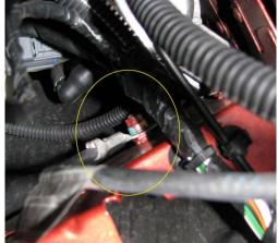
With the earth strap moved you can now drop the new battery tray onto place, the bolts for this will already be fitted with the plastic spacers underneath. Simply line up the three bolts and tighten down securely.
