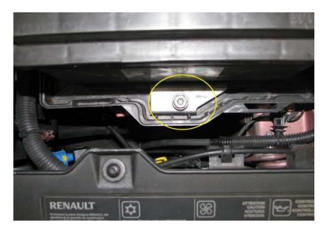
Be careful when you remove the battery, this is heavy so if necessary get someone to give you a hand lifting it out of the engine bay.
