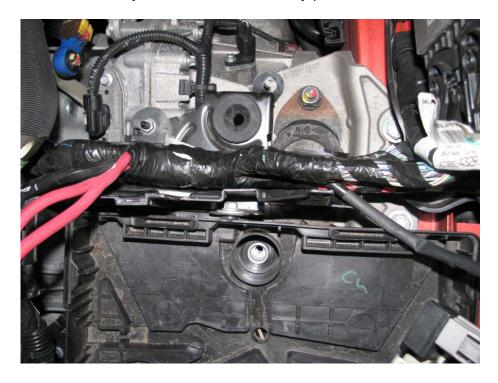
With the harness liberated from the battery tray, remove the three bolts holding the tray in place and lift it out of the engine bay.
