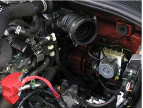
With the hose repositioned you can now drop the airbox in place, insert the filter outlet into the turbo hose, tighten up the hose clip and strap down the nose of the airbox.
