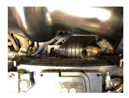
Next the new air filter box can be fitted into the silicone air filter hose and placed into the semi circle cut out in the air box bracket. Once this is done the elastic retaining strap can be fitted around the snout of the air box to hold it securely. The 2 x hose clips can then be tightened around the air filter hose making sure there in an airtight seal and the hose is not deformed in any way.
