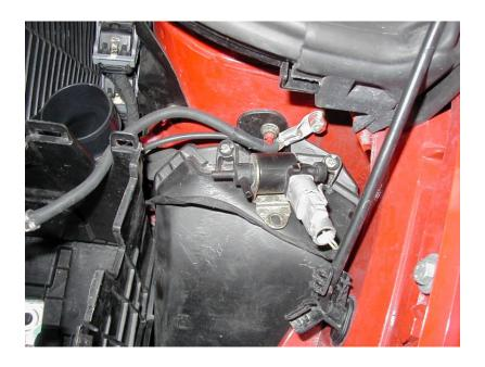
Remove the solenoid mounting bracket by undoing 2 x torx t25 screws, once the bracket is out of the way the torx screws can be refitted using one on them to secure the redundant solenoid in a convenient position.
