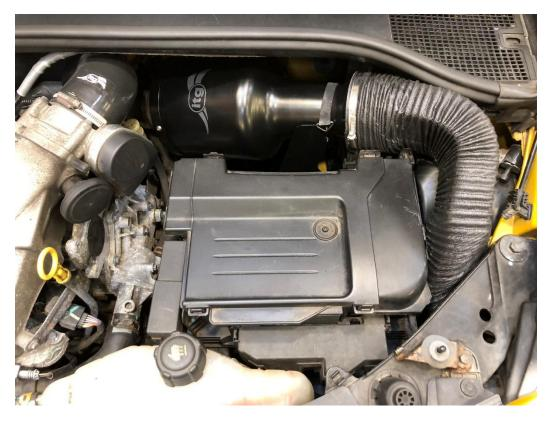
The air box installation is now complete, and the battery can be fitted in a reverse procedure is which it was removed.
