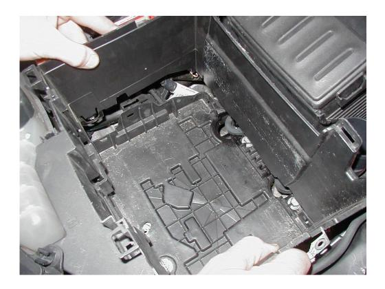
Now with the battery surround still elevated, pull the air box up and out of its rubber mounts and remove it from the car. This may be tricky due to the size of the box so a second pair of hands may be required.
