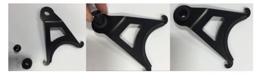
3. Mount the support bracket to the vehicle using the existing mounting stud and secure to the pipe using the rubber strap supplied.
