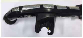
2. Refit the grommet to into the mounting hole on the new bracket then slide in the metal spacer as shown in the picture below. This will allow the OEM bolt to be re used retaining the engine cover fixing location.
