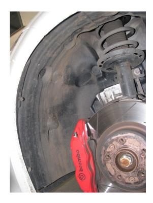
The arch liner is held in place with five push in plastic bungs and two torx screws at the front of the wheel arch, remove these and then carefully wrestle the liner out.
