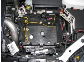
Now remove the battery, disconnect the negative terminal first followed by the positive, then remove the black metal strap that holds the battery in place and lift the battery out.
