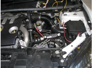
With the hose positioned as shown above you can now fit the aluminium pipe between the silicon hose and turbo intake hose. The pipe should be fitted so as the logo is visible and the correct way up.
