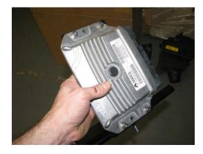
You can now fit the new battery tray and ECU into the engine bay. You may find that the front brake pipe on the brake master cylinder fouls the back of the ECU, if this is the case VERY carefully bend the pipe until it clears by 2-3mm.
