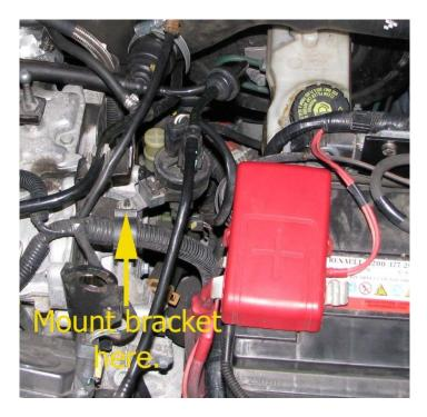
Two p-clips are provided to attach the wiring harness to the top of the ECU mount along with a couple of cable ties if they are needed.
