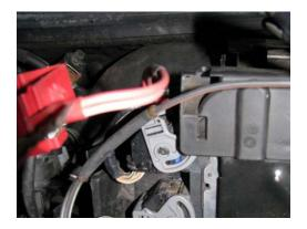
Finally you are ready to remove the airbox, slacken off the hose clamp connecting the airbox to the inlet hose and pull the hose away from the airbox. The airbox is mounted on push in rubbers, so it's just a case of giving the airbox a good hard tug to remove it – removing the air feed pipe first may also make things a little easier.
