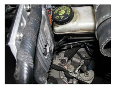
You can now plug the ECU back into wiring harness ensuring that the grey latches are fully down and secure.
