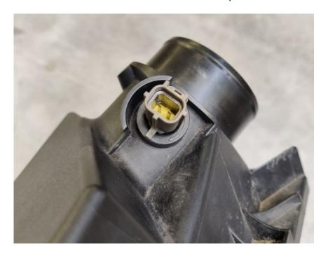
6) Place the temperature sensor into the new ITG pipe in the orientation shown below & twist this (clockwise) into place to lock the sensor into the boss.
