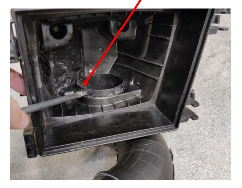
7) Finally remove the airbox mounting grommets from the car – you are now ready to fit your new ITG induction kit.
