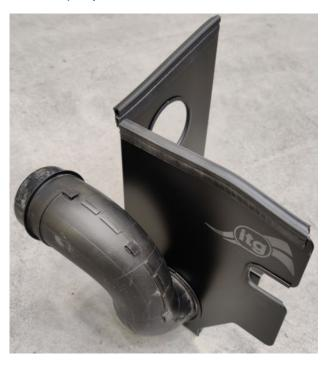
2) Place the heat shield and duct into the engine bay and line up the duct ready to slot back into the OE front scoop. Ensure the bonnet cable is located in the cut-out on the heatshield as shown.
