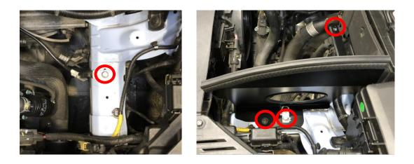
Step 2: Fit the airbox by inserting the inlet side into the hole in the mounting bracket then insert the filter neck into the existing intake hose, this can be secured by tightening the hose clamp. The Final bolt can then be tightened.
