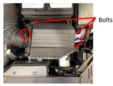
Step 3: Remove the scoop by removing the two bolts securing the scoop to the slam panel using a 10mm socket. (Keep these bolts safe as they will be used to refit the mounting bracket).
