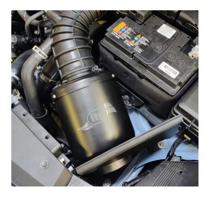
4) Re-tighten the hose clamp on the end of the OE hose (10mm socket)
