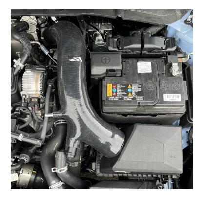
5) Connect up the 2x ancillary hoses to the main hose & re-seat the hose clips over the spouts.
