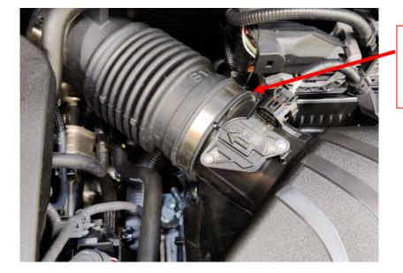
Head of the hose clip is located underneath and facing towards the rear of the car.
