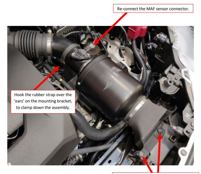
Push the 2x trim clips through the scoop's mounting flange and back into their original locations in the car's chassis.
