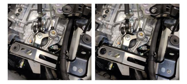
2) Connect the supplied connector blank to block off the vac solenoid plug.
