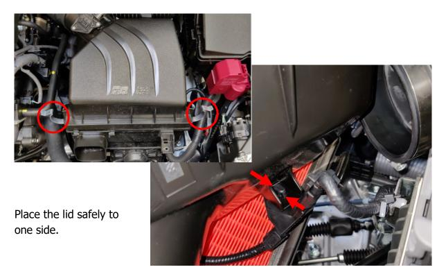
8) Pull the vacuum hose off the lower half of the airbox and turn the airbox upside down, to reveal the wiring clip holding the connector for the solenoid. Once removed, place the airbox base safely to one side.
