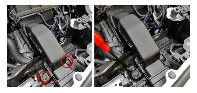
2) Pull the front of the scoop upwards and pull it out of the lower airbox.
