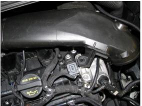
If you then remove the right hand section you will have good access to remove the oil breather pipe that connects the crossover pipe to the cylinder head.
