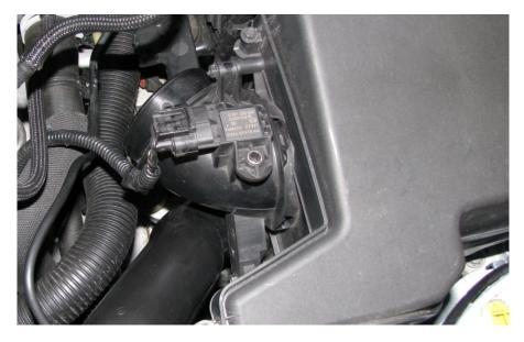
With the sensor out you can now start to pull out the rest of the system, first unclip the pipework connecting the airbox to the slam panel. The airbox is mounted on rubbers so there is enough movement to pop the pipework out. Then disconnect the flexible hose connecting the airbox to the engine crossover pipe and you're ready to lift the airbox out. This is mounted on push in rubbers so, with a bit of force, will lift straight out.
