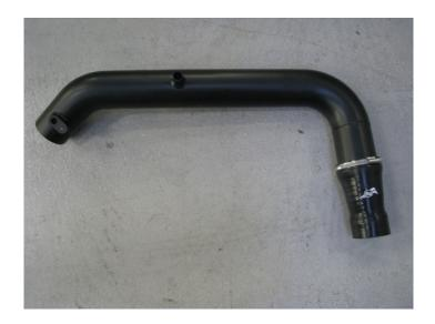
The logo on the hose should always be in the same place so if you align as shown above, you should have the correct orientation - looking at the pipe end on, it should be as below.
