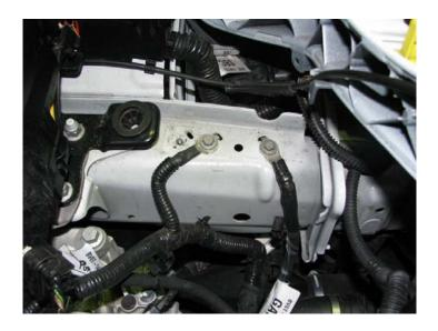
You can now drop the airbox into place, feed the duct through the gap alongside the radiator that goes through to the nosecone and bolt the bracket into place ensuring that the earth straps are reconnected (be aware that one of the bolts is M6 and the other is M8).
