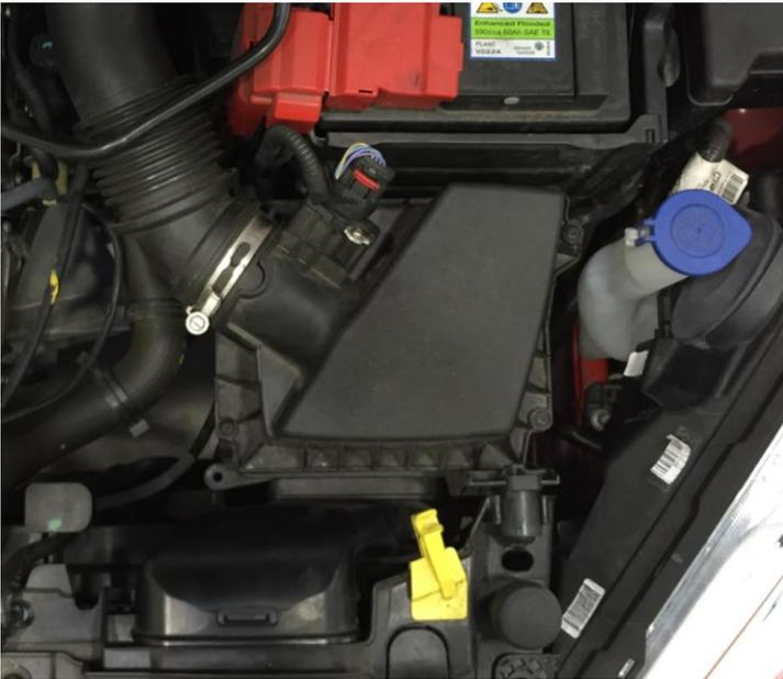
Removing stock airbox. Gently disconnect the MAF sensor, remembering to depress the red safety latch. This will allow the plug to be removed correctly, before loosening off the hose clip that connects the air-box lid to the inlet.
